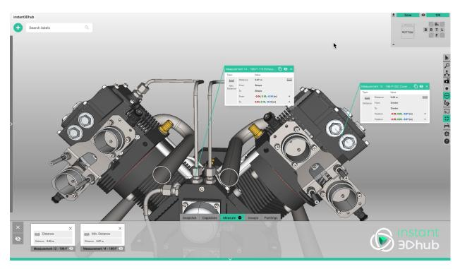
• Arc Measurements: Arc measurements are defined by three points in the 3D Space, typically derived from surfaces of the geometry. They provide information on center, diameter, circumference, angle and axis of the respectively defined arc.
