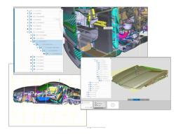
Clipping rooms or clipping volumes are defined by a combination of six planes. As for clipping planes, they can be derived from nodes of the InstanceGraph interactively, for example using the volume of a node.
