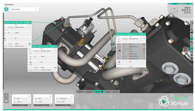
• **Double Measurements**: Double Measurement provide information on relations between topological entities e.g., distances or angles. For convenience, the result set automatically matched for the input data types.
